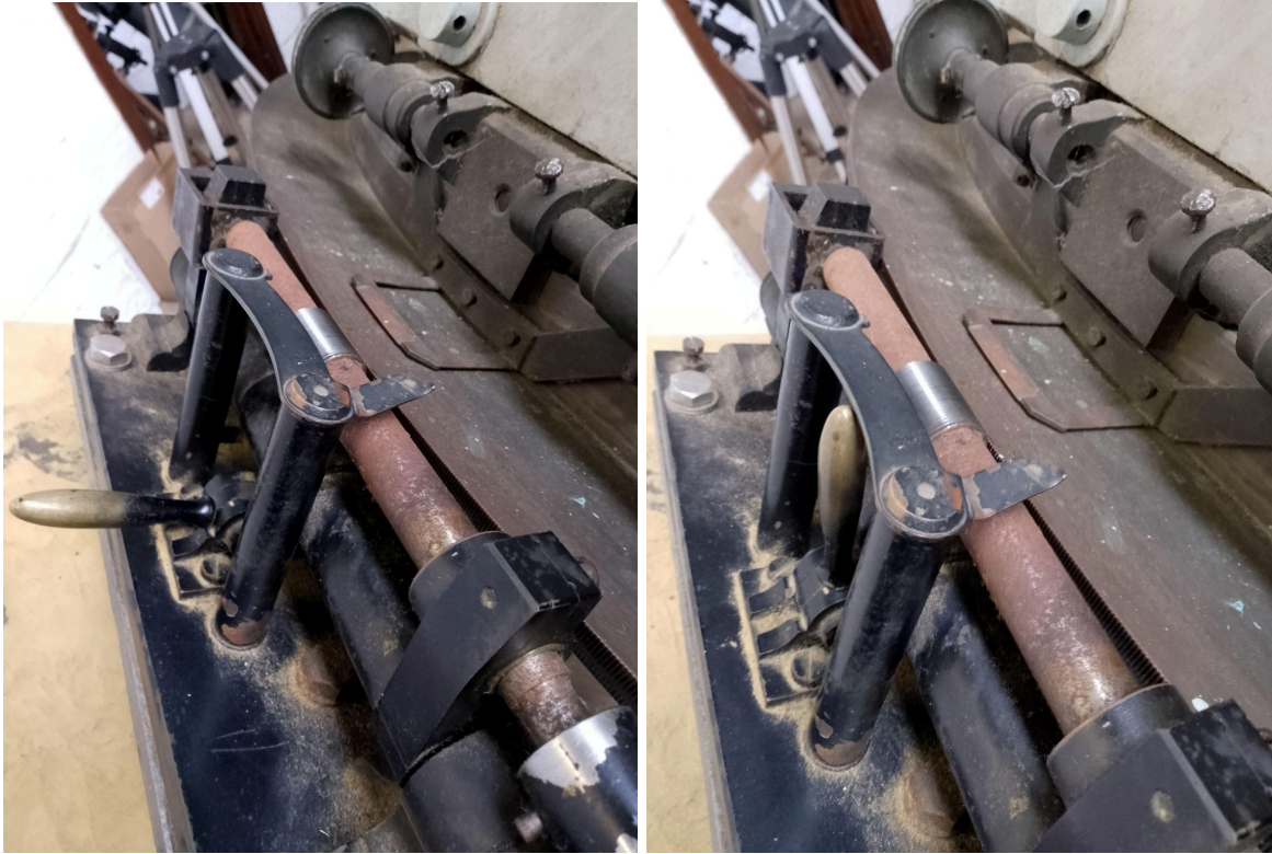
The worm gear and lever, showing it both disengaged (left) and engaged (right). Make sure it is always left disengaged, except when the motor drive is engaged
