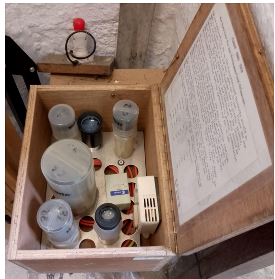
The heated box of Meade Plössl eyepieces, containing: 40mm, 36mm, 32mm, 25mm, 15mm, 12.5mm
