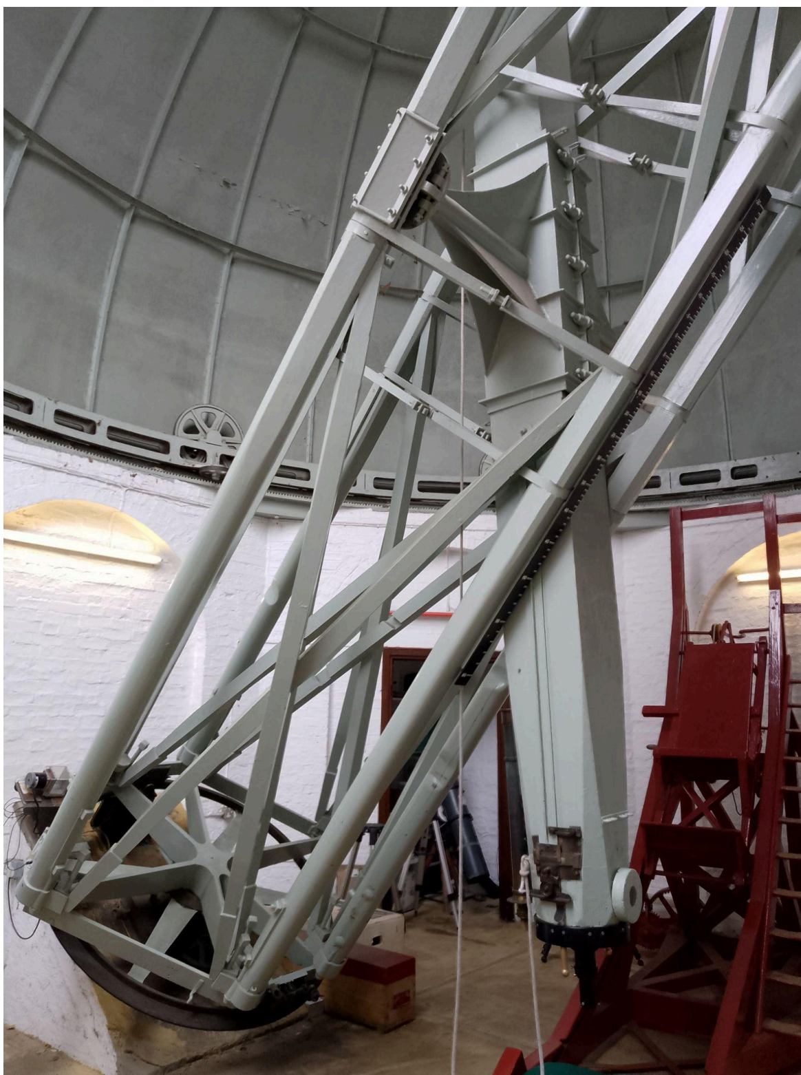
The Northumberland telescope in its vertical resting position, showing the declination meter on the side, along with the ObsChair and storage alcove in the background.
