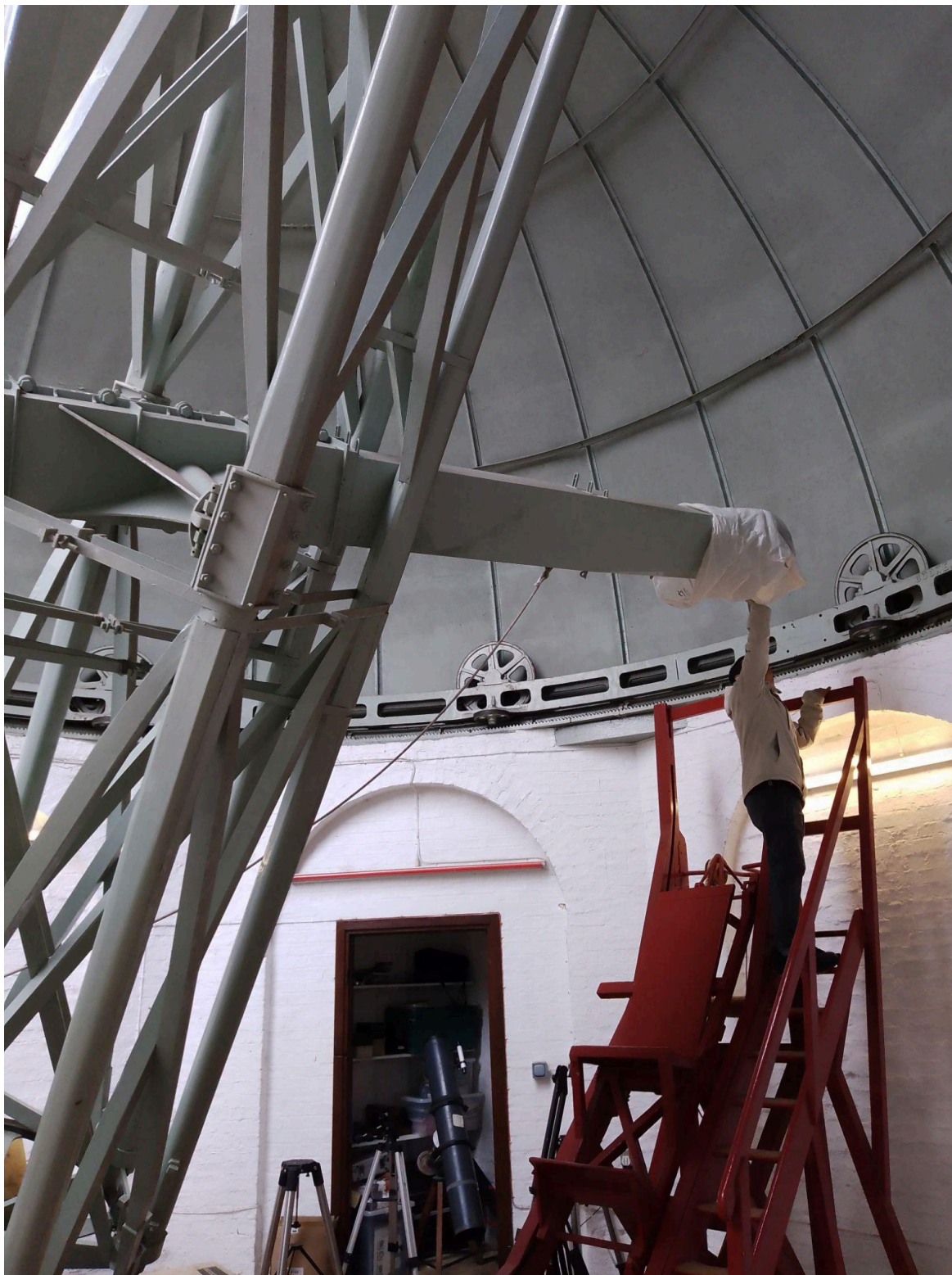
Photo demonstrating how to remove/replace the lens cap on the Northumberland.
